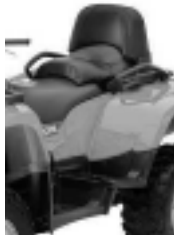
An ATV designed to carry a passenger has a separate seat, handholds and footrests.
