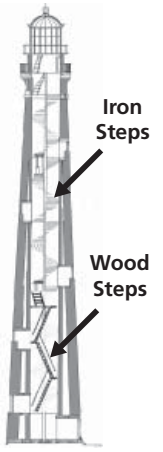
Repairs to the steps may have looked like this
