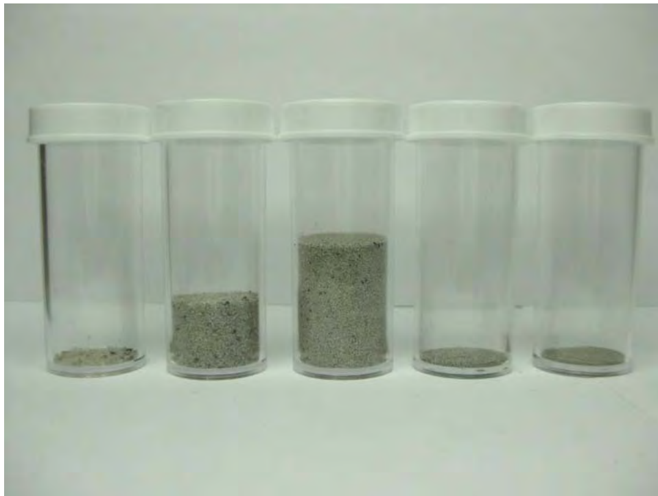
Figure 4: Photographs of the graded sand separated from mortar samples CALO.Mortar.1 (top) and CALO.Mortar.2 (bottom). The sands are both narrowly graded with a vast majority of material found between the No. 30 and No. 100 sieves.
