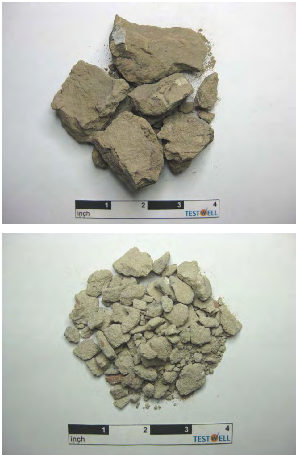
Figure 1: Mortar samples CALO.Mortar.1 (top) and CALO.Mortar.2 (bottom) received by Testwell for comprehensive analysis.
