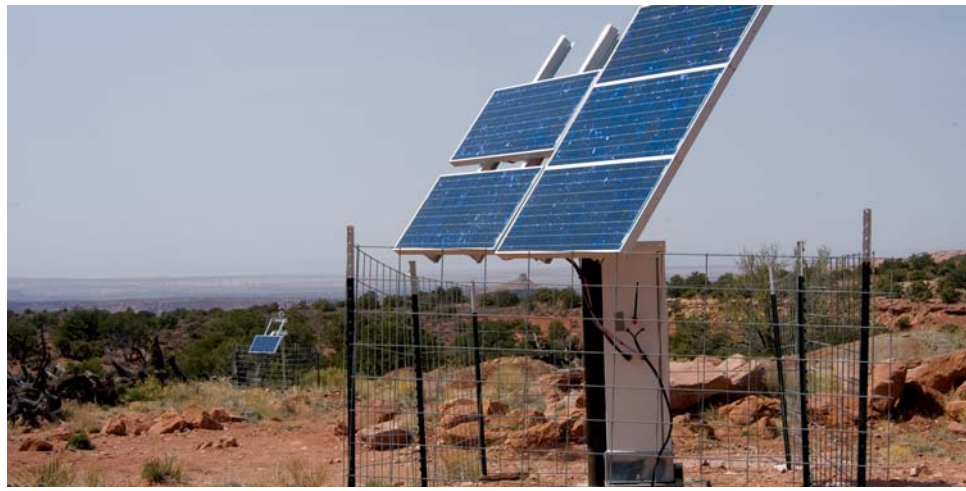
A small footprint: a few solar panels power the seismic stations and the satellite dish that transmits the data they record.
