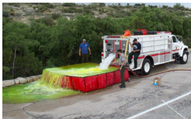
Waylon Cox, Stan Allison and Tilo Garcia mix freshwater with fluorescein dye that was then allowed to flow into Bat Cave Draw. (NPS Photo by Paul Burger)
