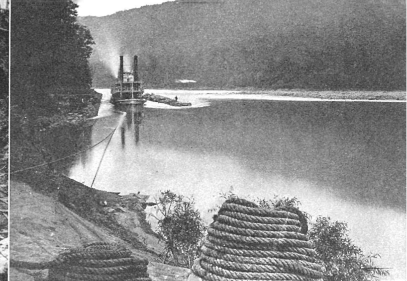
After the fall of Chattanooga, supplies were brought to the Union Army by steamboats. It was necessary to warp the boats up the river through rapids. (Signal Corps, U. S. Army)
