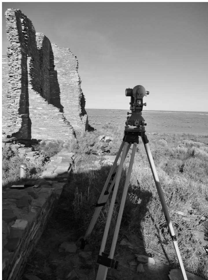
Figure 102. Theodolite survey of Pueblo Pintado's west wall
