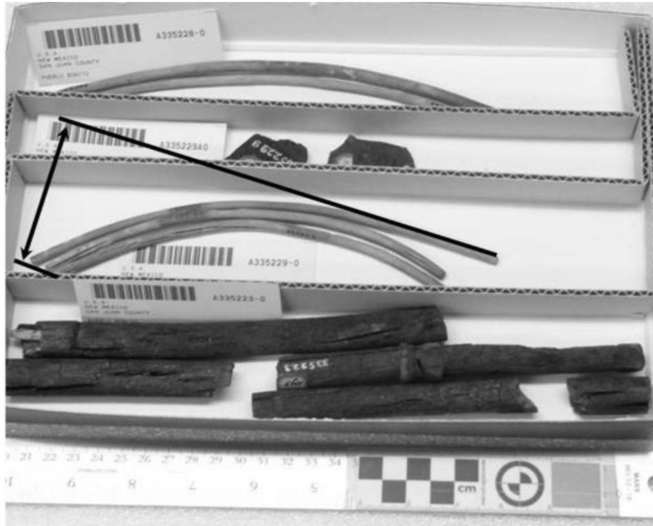
Figure 105. Five bow shaped pieces of wood in the Smithsonian collection The black lines and arrow indicate the “offset” dimension measured for each.
