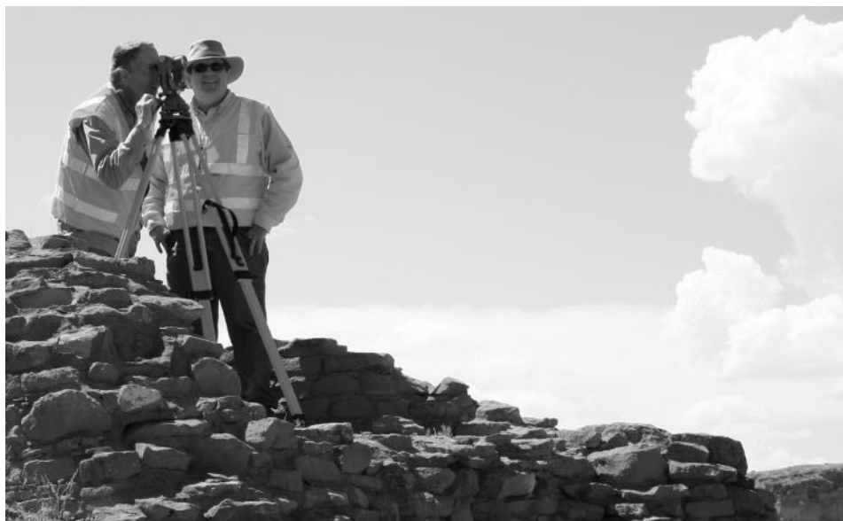
Figure 42. Theodolite position at Casa Chiquita for survey of east horizon
