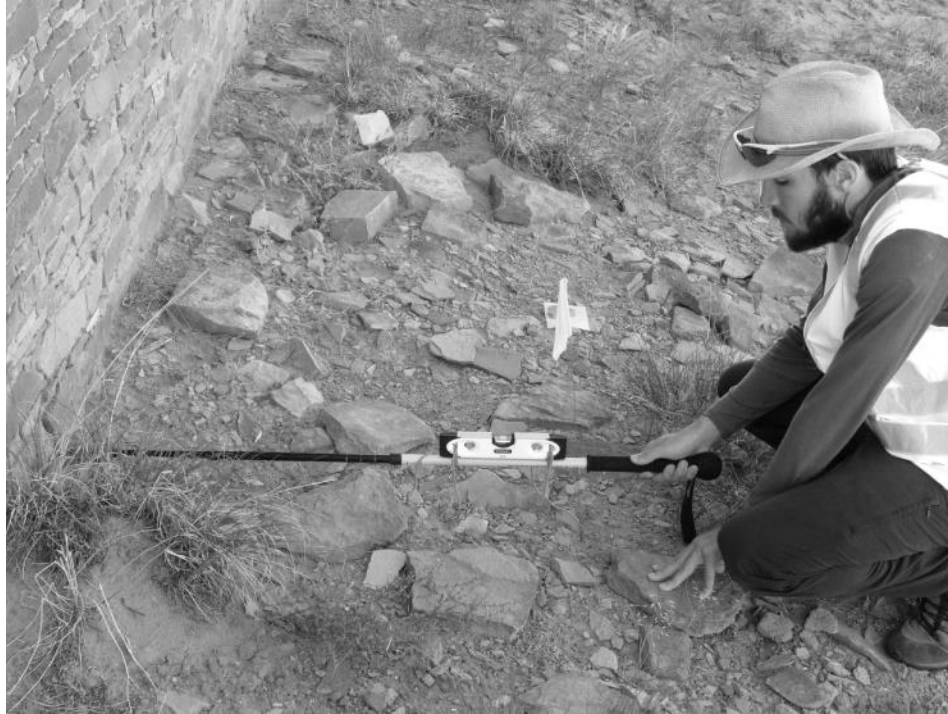
Figure 25. Improved angle measurement technique for walls
