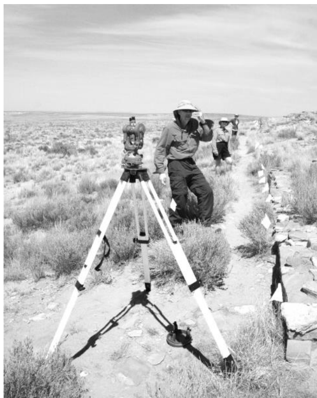
Figure 62. Theodolite survey of Pueblo Alto's north wall, west section
