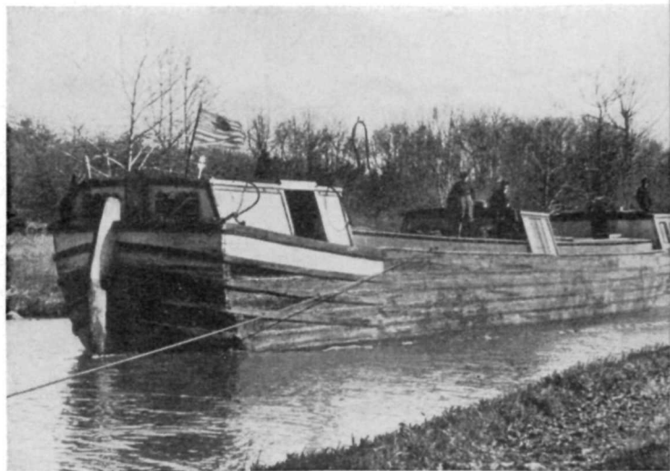
A typical canal boat. An extra mule team was carried in the forward cabin. The small structure in the center of the boat was the "hayhouse" where the mule feed was kept. The captain and his family, or the hired crew, lived in the aft cabin. Underwood and Underwood Photo.
