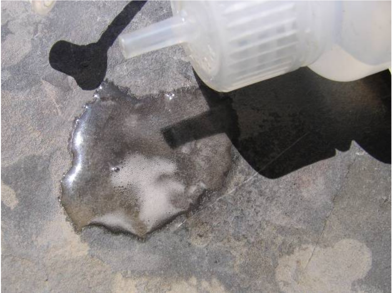
Figure 7.5 Limestone reacts with acid, even weak acid. Here, diluted hydrochloric acid is dripped on a block of limestone, causing it to fizz (carbon dioxide is being released).
