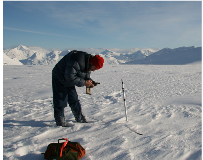
An NPS researcher records a GPS waypoint at an exposed mass balance stake on the Harding Icefield in Kenai Fjords National Park.
