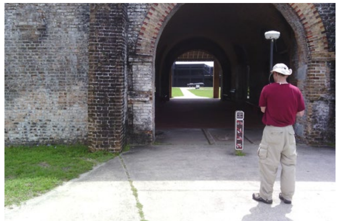
Figure 6.5. Image of rover GPS data collection at the Sally Port of Fort Pickens at Gulf Islands National Seashore as part of the vulnerable asset elevation project in 2015.
