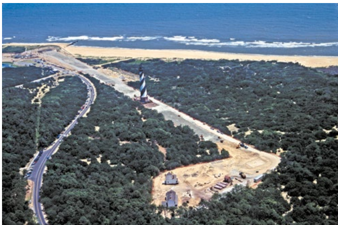
Figure 8.10. In this example of relocation and retreat, the Cape Hatteras lighthouse was moved inland using a railway. Photograph by NPS.
