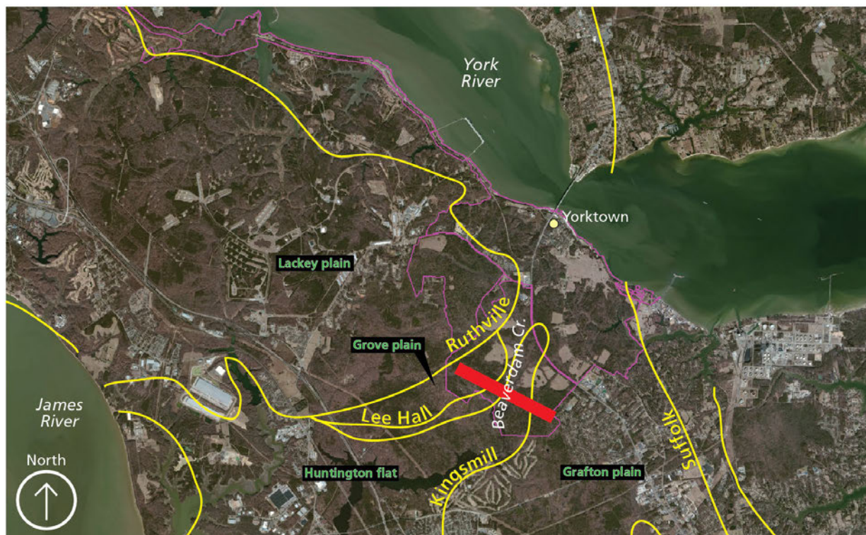
Figure 19. Map of generalized groundwater flow through hydrogeologic units at Yorktown Battlefield. Red line on aerial image is the general trace of the cross section. Yellow lines indicate scarps (see figs. 3 and 4); pink line is park boundary. Orange and yellow unit colors correspond to units on the geologic time scale. Graphic is not to scale and is vertically exaggerated. Note the discontinuous nature of the perched Columbia aquifers and Cornwallis Cave confining units due to the presence of the step-wise riverine scarps and incision of Beaverdam Creek. The Yorktown-Eastover aquifer is completely buried throughout the battlefield area. Graphic is adapted from Speiran and Hughes (2001, figure 11) with information from Johnson (2007) by Trista L. Thornberry-Ehrlich (Colorado State University).
