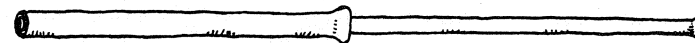
The blowing iron for giving the glass its hollowness and its general form
