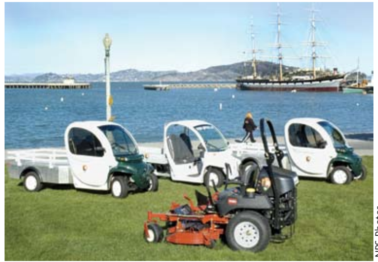
Utility trucks are powered by electricity and the park mower runs on 100% biodiesel.
