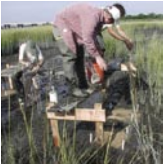
Left: Researchers determine the surface elevation of the wetlands before sediment is applied to raise the level of the marsh.
