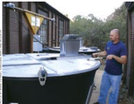
Organic materials such as food scraps, lawn clippings, and shredded paper turn into compost using an Earth Tub.
