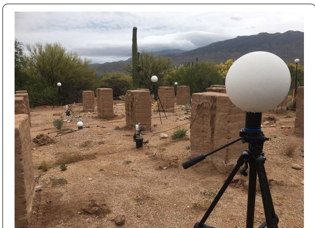
Fig. 4 LiDAR scanning equipment and test walls during Epoch II. Photo NPS/Alice W. Biel
