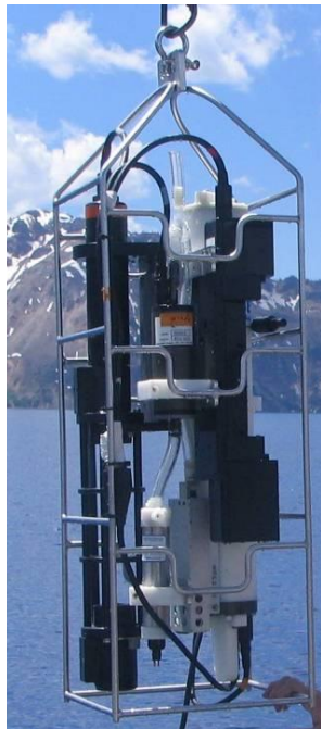
CTD package used at Crater Lake. Tall black sensor on left is transmissometer. (NPS photo)
