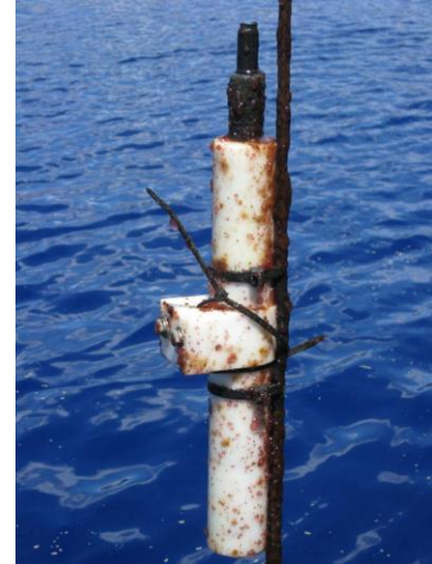
Recovering a SeaBird Electronics temperature sensor after a year in the Crater Lake water column (NPS photo)
