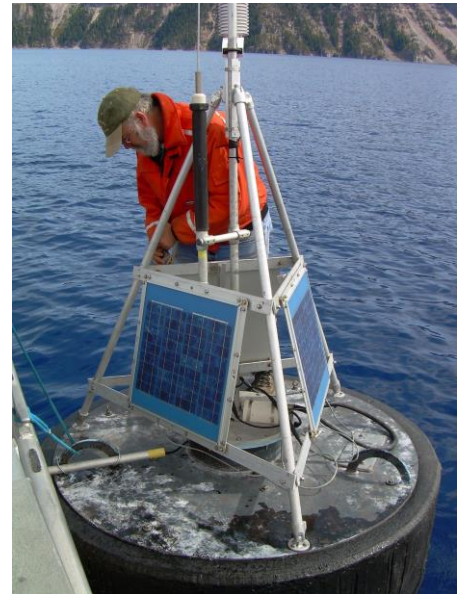
Dr. Robert Collier (Oregon State University) working on the floating weather buoy. The temperature sensor used for tracking onset of stratification is located under the buoy at a depth of approximately one meter (NPS photo).
