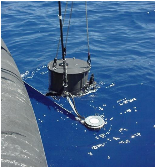
Two of the meters used to measure light penetration in Crater Lake, Kahl photometer in the foreground and the Licor behind (NPS photo).
