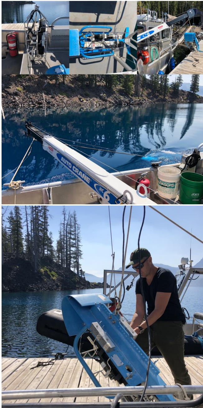
Equipment and setup of CTD sensors for a near shore tow along the shoreline of Crater Lake (NPS photos).
