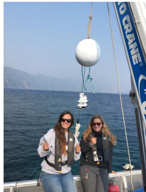
Underwater mooring with high frequency sensors attached. Deployment and collection requires the use of the research vessel crane (NPS photos).
