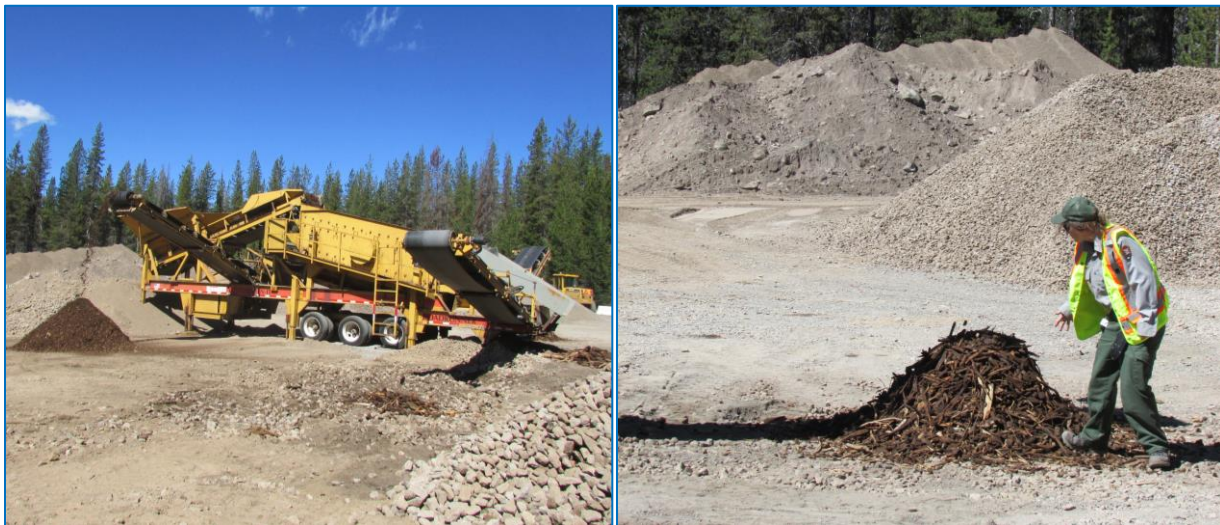
Figure 7. A screen plant was used to sort readily compostable materials (left) from partially composted woody debris (right) to augment conditions at disturbed sites. Photos by Jen Beck.
