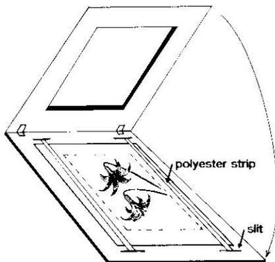
4. Turn the board face up. Place the object on the board, and gently insert first one side and then the other under the strips, centering the paper in the space provided.
