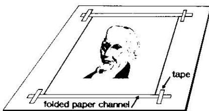
5. Cut a window mat that covers the paper channels and hinge it to the back mat on the inside with tape for framing.
