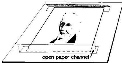
4. Close the paper channels and tape them to the mat board, placing the tape vertically across the ends of the channels. Allow space between the tape and the mounted object, for example, about 1/16th inch for a letter-sized object, and slightly more for a thicker or larger object.
