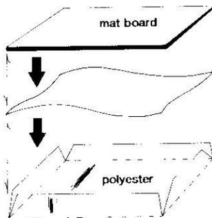
4. Center the object to be mounted face down on the polyester. Place the mat board on top. Weight the mat board. Fold over the polyester flaps along two adjacent sides and tape them to the back of the board with double-sided or archival tape. Remove the weight and check for the proper positioning of the object. Tape the other two sides.
