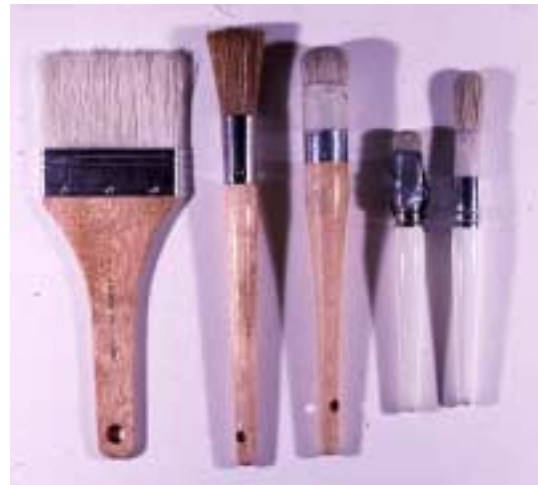
Figure 1. Assortment of brushes, from l. to r.: new paint brush, large new stencil brush, large stencil brush after heavy use, stencil brush after heavy use, stencil brush after light use.
