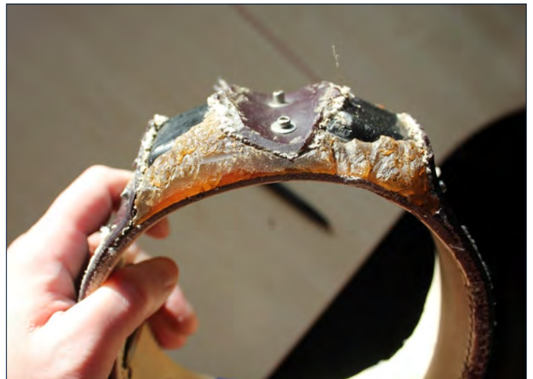
Wolves are very hard on collars. These photos show damage sustained on retrieved collars. NPS Photo / Kajja Klauder
