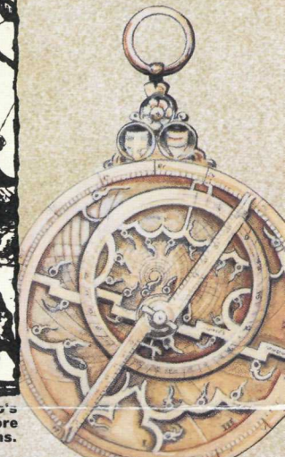
Sixteenth-century navigators used the astrolabe to find latitude.
