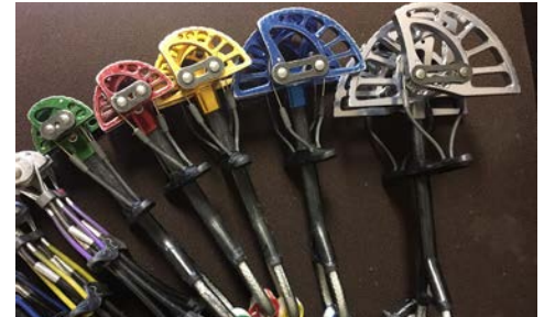
Temporary anchors used by climbers are reliable and removable. NPS
