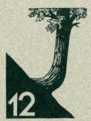
Don't build a house where you see trees like this one! The soil on this steep slope tends to slip downward. and the movement would eventually topple a wall, telephone pole, or other nonliving object. But a tree, if the tilting is slow enough, keeps trying to straighten up as it grows, resulting in a curved trunk
