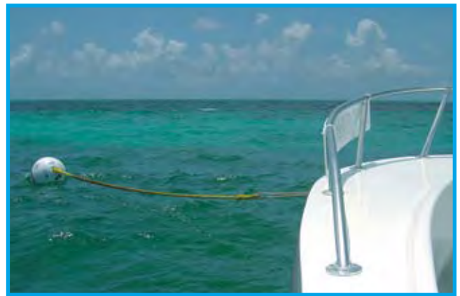
Mooring buoys provide an alternative to substrate-damaging boat anchors. Photo by FKNMS.
