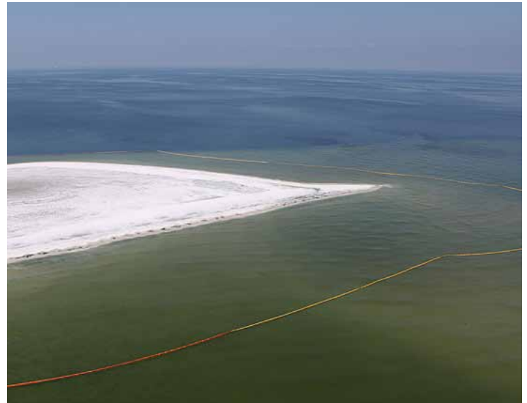
Booms in place around Cat Island, Gulf Islands National Seashore, in an attempt to keep oil from reaching the shoreline
