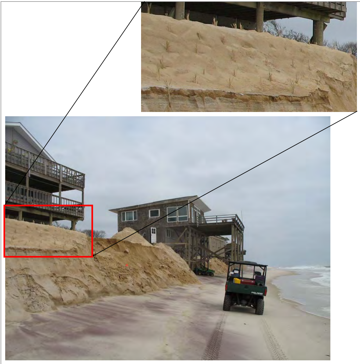
Figure 4. Photo showing dead vegetation (inset) on eroding replenishment material at Fire Island. Photo: Rachel Hehre, April 2008.
