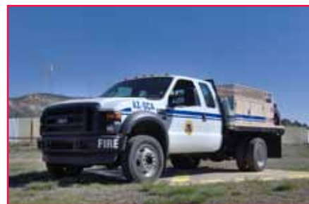
New standardized BIA Model 52 Engines on display at Dulce, NM. Initially started as a grassroots movement, the design and layout of the fleet comes directly from the experience and feedback of the engine technicians and field operators who build and maintain the fleet throughout the Nation. Photo: Dennis Zentz, BIA Model 52 Program Manager, Dulce, NM, 2009.
