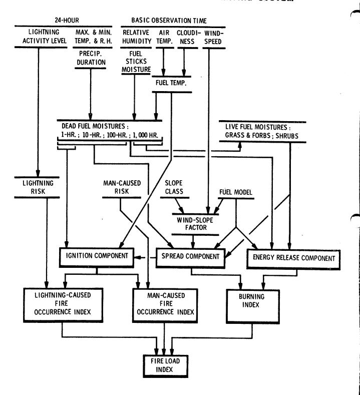
Figure 2. -- Structure of the 1978 National Fire-Danger Rating System.
