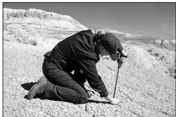
Figure 11. Erosion stakes being installed perpendicular to the surface at Fossil Butte National Monument in 2002. Measurement and documentation of movement of the erosion stakes provides information on local erosion rates and the stability of in situ paleontological resources. National Park Service photograph.
