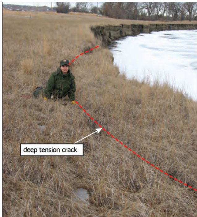
Figure 14. Photograph of the south bank of the Missouri River. Deep tension cracks (dashed red line) have developed approximately 2 m (7 ft) from the bank's edge. Ultimately, bank failure will occur along this tension crack. National Park Service photograph taken on 9 March 2007 shortly before ice-out. Photograph from Ellis (2008, figure 4.3).
