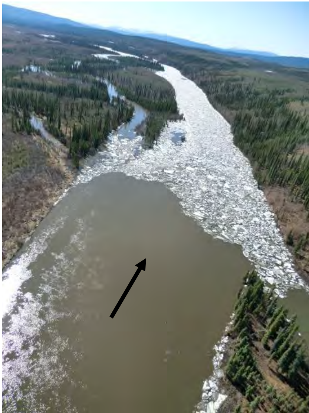
Figure 128. Ice jam on the Kobuk River near the proposed northern crossing on May 29, 2013.
