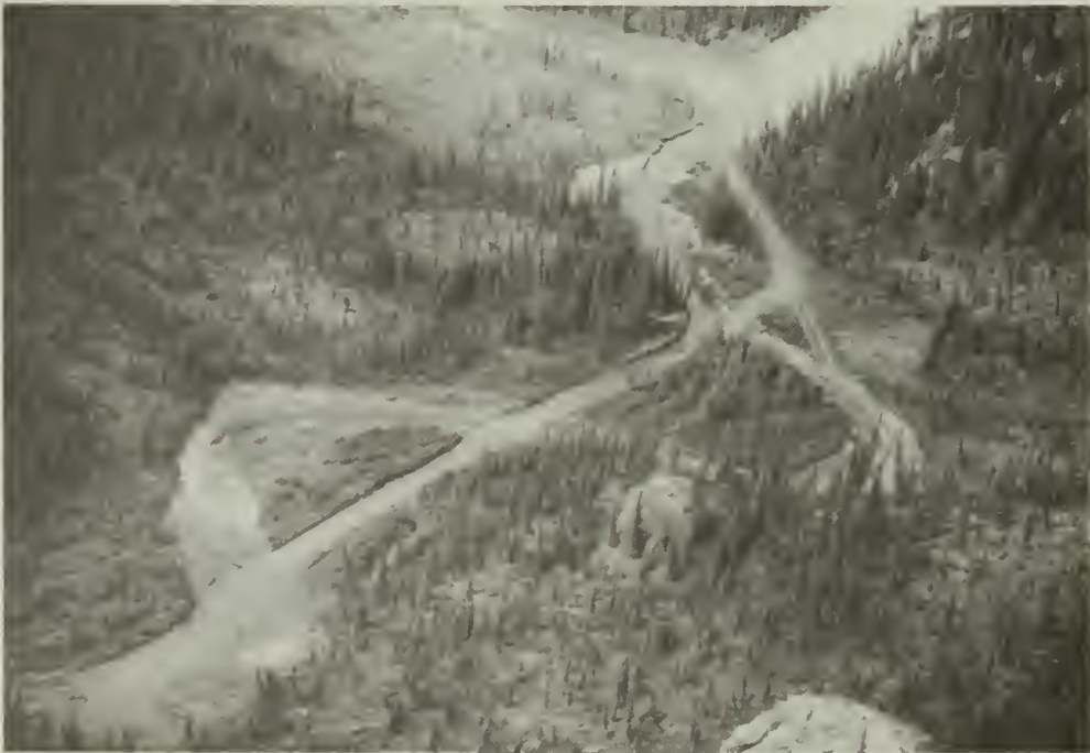
Illustration 14. Stream channel in lower Mascot Creek has been diverted from its natural streambed by construction of access road that crosses natural stream meanders.
