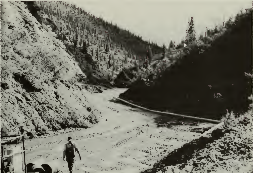
Illustration 12. Stream channel manipulation by placer mining on Mascot Creek has completely altered the natural stream channel in this area. Stream bank sloughing has also occurred on left side of stream channel. Pipeline transports process waters to sluice box located downstream.
