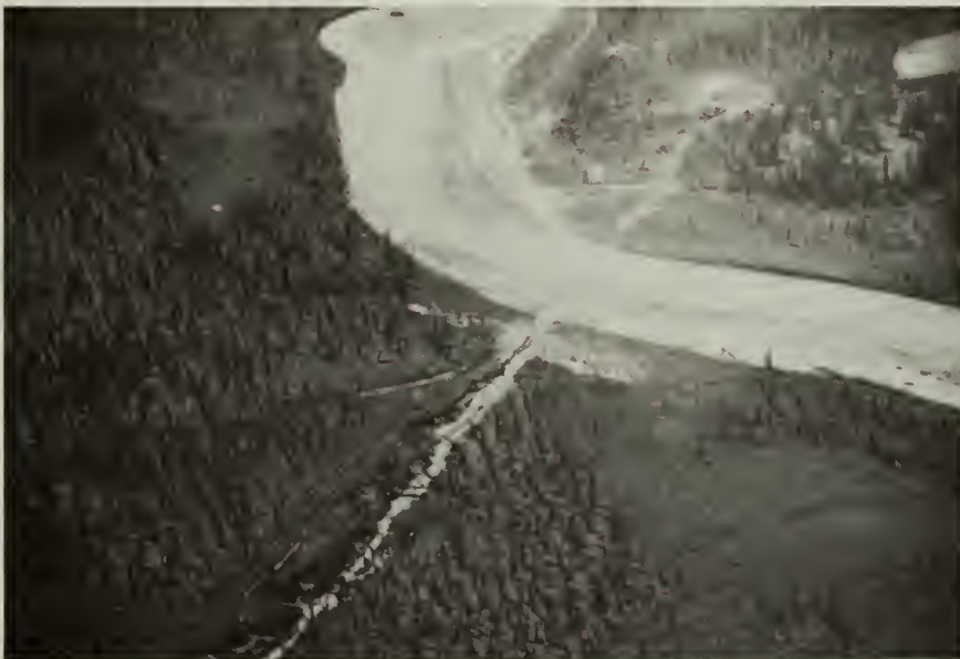
Illustration 6. Severe erosion occurring along winter trail from Wiseman to Mascot Creek. Picture was taken at point where trail crosses Glacier River 3 miles east of Mascot Creek.
