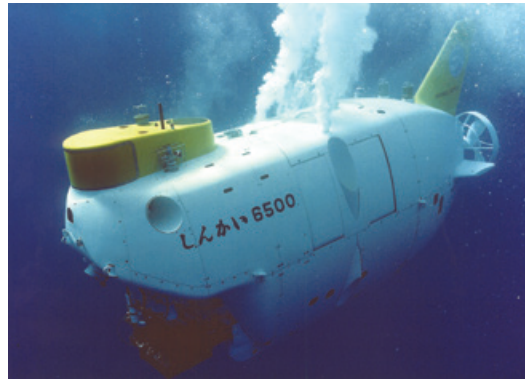
The Shinkai 6500 of the Japan Agency for Marine Science and Technology (JAMSTEC) is the world’s deepest manned research submersible, capable of operating at ocean depths down to 4 miles. It was used in 1999 by Japanese and U.S. scientists to study Lō‘ihi Volcano. (Photograph courtesy of JAMSTEC.)
