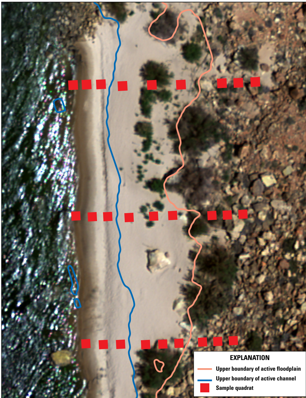
Figure 6. Diagram illustrating the sampling layout for randomly selected sites. Three transects are placed perpendicular to the river channel, and nine 1-square-meter (m 2 ) sample quadrats (illustrated as red squares, not shown to scale) are placed on each transect. Quadrats are stratified by hydrologic zone (active channel, active floodplain, and inactive floodplain). Base image from Durning and others (2016).
