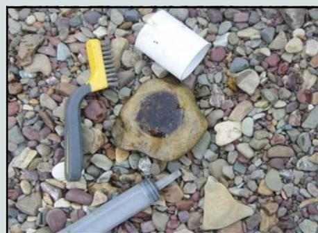
A cobble used to collect periphyton. The algae is scrubbed using a metal brush and rinsed into a collection container. Photo Credit: B. Schweiger
