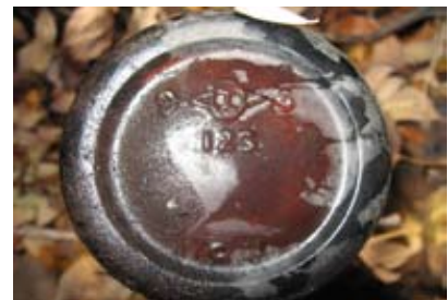
Figure 2. This bottle mark gives us the following information - Plant Code 9 = Streator, Illinois; year code 3 = 1933. The 123 is a code for the particular bottle mold used (Toulouse, 1971, p. 403).
