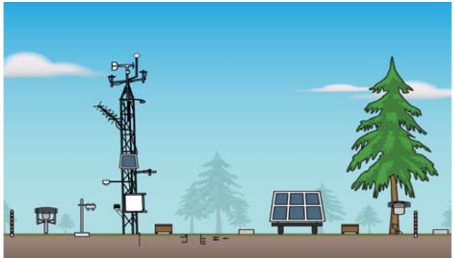
Figure 2. Instrumentation General Schematic; from left to right: snow stake, Geonor precipitation sensor, net radiometer, tower, battery enclosure (brown box), soil temperature and moisture sensors, runoff collector (small gray box), solar panel, enclosure, tree sap flow and point dendrometer, under canopy snow stake and another runoff collector. On the tower are (top to bottom): wind direction/speed, lightning rod, quantum sensor and pyranometer, PTZ webcam, Yagi antenna for AFAR radio, solar panel, NDVI sensor, ultrasonic snow depth sensor, datalogger enclosure (white box) and air temperature/relative humidity sensor.
