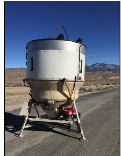
Hopper used to distribute seed over burned area.
