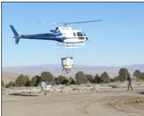
Helicopter returning with empty hopper after seeding.
