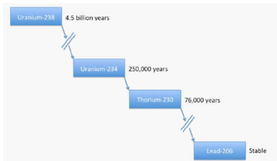
Figure 1. A simplified version of the uranium-238 decay chain. The number next to each isotope indicates its half-life – that is, the time after which half of a given number of initial atoms will remain. The double lines indicate that intermediate decays have been removed for clarity. Though the intermediate daughter isotopes have shorter half-lives than uranium-238, they are continuously resupplied by decay of isotopes farther up the chain. The current results indicate that sufficient time has passed for thorium-230 and uranium-234 to be in equilibrium with uranium-238, which requires at least 1 million years.
