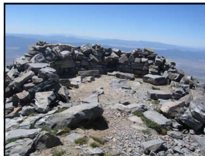
This stone cairn (L) marked one of the azimuth directions for instrument readings and calculations. The circular rock structure (R) was over four feet high with a tent inside to house the 1881 survey instruments. Photos by K. Jageman.
