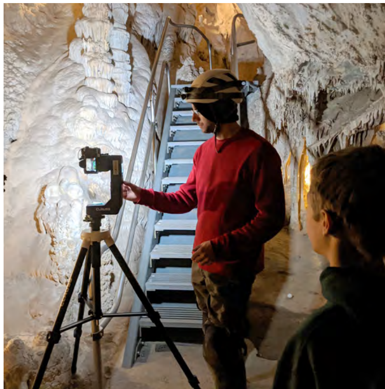
Caption: Blase LaSala prepares for the LiDAR and color scanning of part of the Lehman Caves tour route. This 3D scanning resulted in a virtual tour of the cave, available on the Park's YouTube channel.
