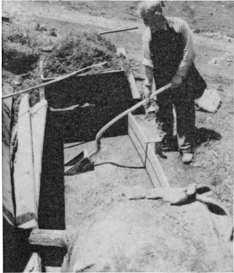
After the bark is shredded, it is placed in a tanning vat. Here it is being dipped with a wooden strainer before the "ooze" is renewed with fresh bark
