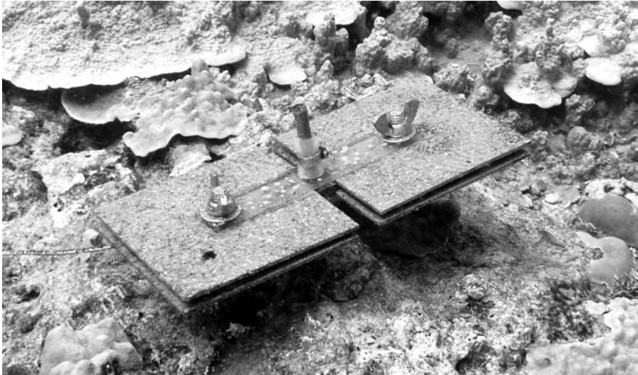
Figure 1. Recruitment sampling apparatus, "plate unit." Photo by Ian Lundgren.
