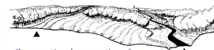
Cross-sectional perspective of Confederate (concrete) and Union (asphalt) avenues along siege line. (Deb James, HAER 1997)
