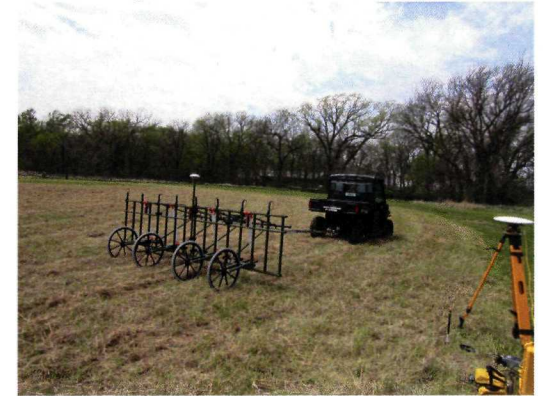
SENSYS magnetic gradiometer array towed by a UTV. A GPS base station is in the foreground. NPS photo
