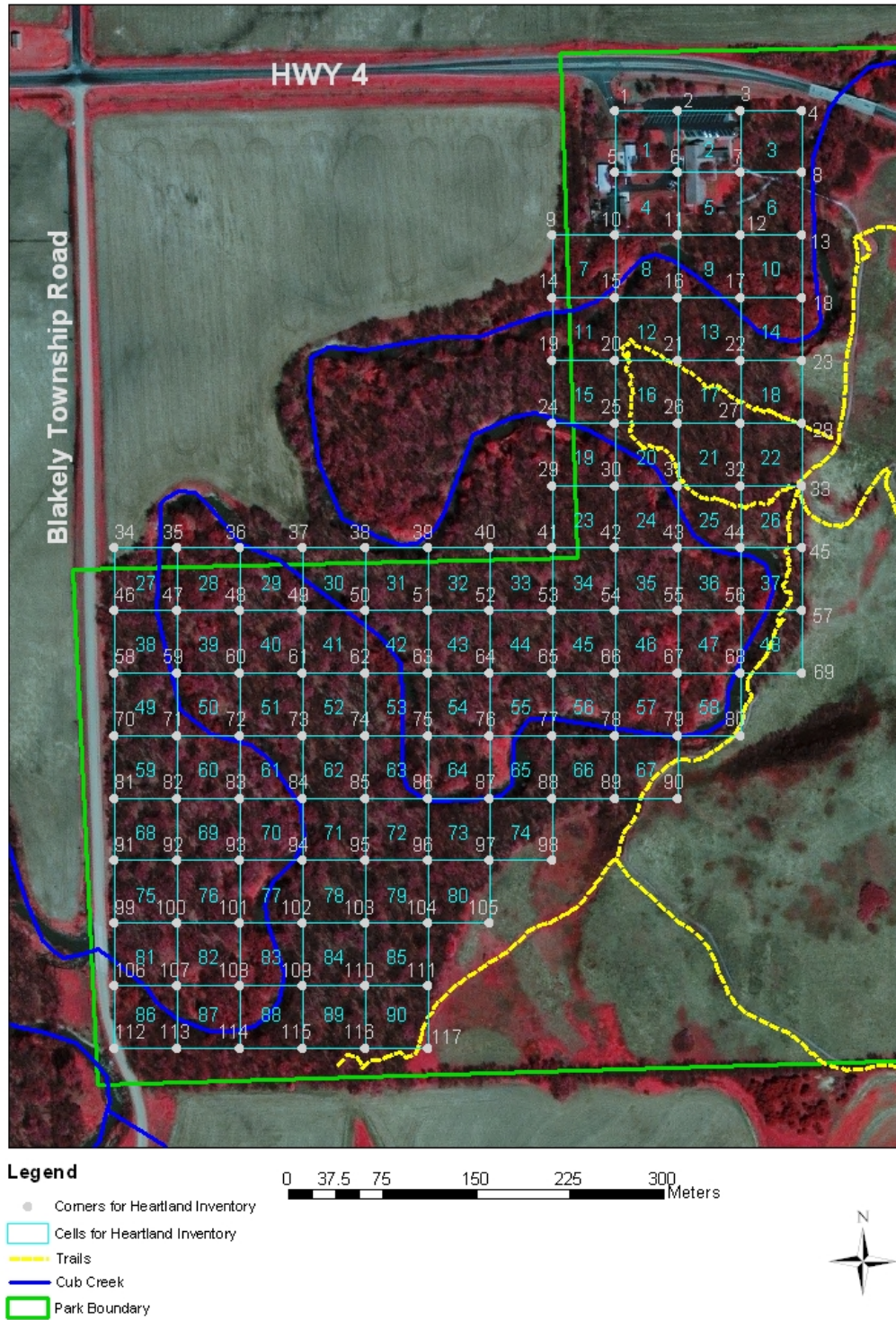
Figure 2. Sample grid (cell size = 50m x 50m) used to select random search areas. Cell ID number is in the center of each cell. Grid vertex numbers are labeled above each vertex.
