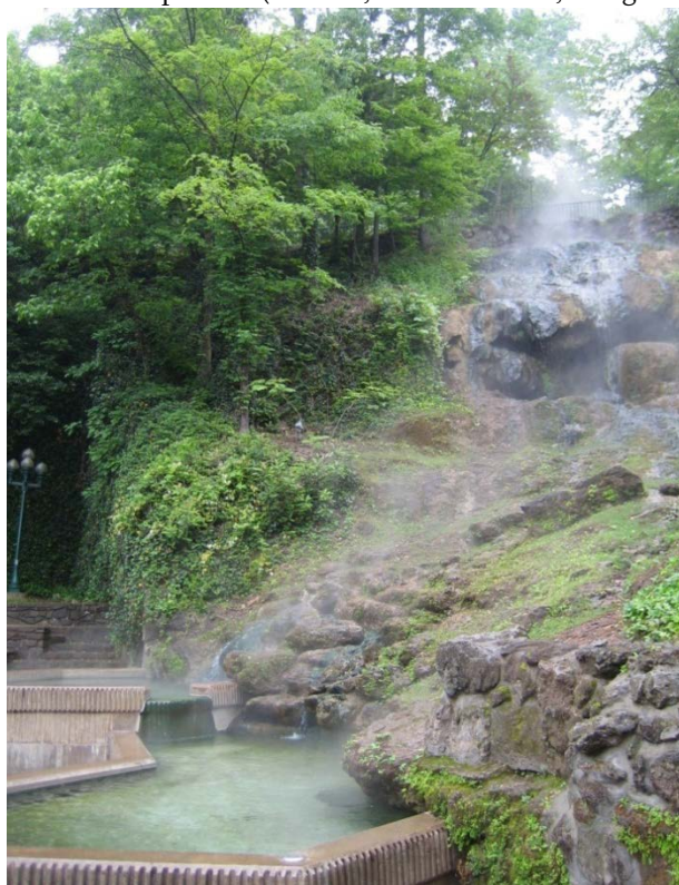
Figure 10. Hot Water Spring Cascade. The park supports a 12 to 15 m (40 to 50 ft) flowing display spring at Arlington Lawn to demonstrate how much of the entire hillside might have appeared if the hot springs were still flowing freely. The feature is plumbed to mix hot and warm waters to a safe temperature, and blocks of tufa were put in place to resemble a natural flowing hot spring. Photograph by Trista L. Thornberry-Ehrlich, taken in 2007.
